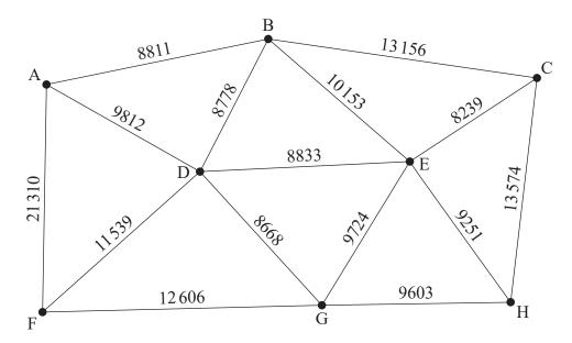
The computer network could be designed such that each building is directly connected to at least one other building and hence all buildings are indirectly connected.
